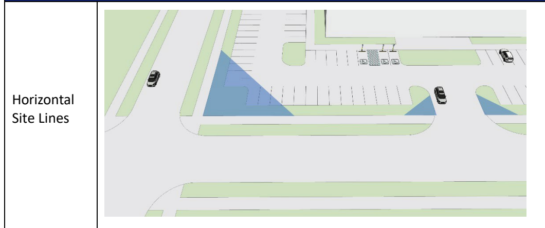
Figure 4-4, Vertical Site Lines and Horizontal Site Lines
